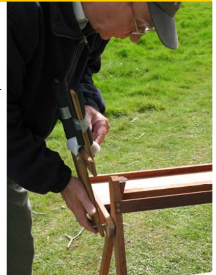
Attach the model holders which are stacked up under the Transmitter shelf. They are adjustable for width.
