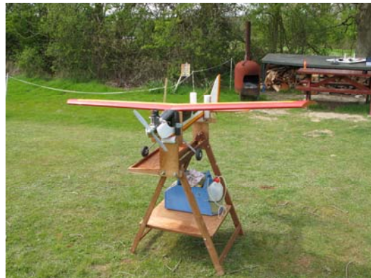
Do ensure you place your model box on the bottom shelf to stabilise the stands.
